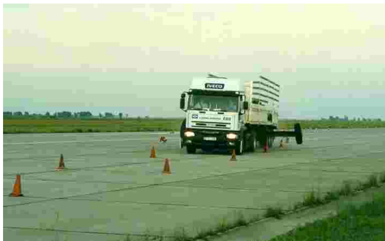
Figure 3. Path of single lane change for the drive tests of KTI.
