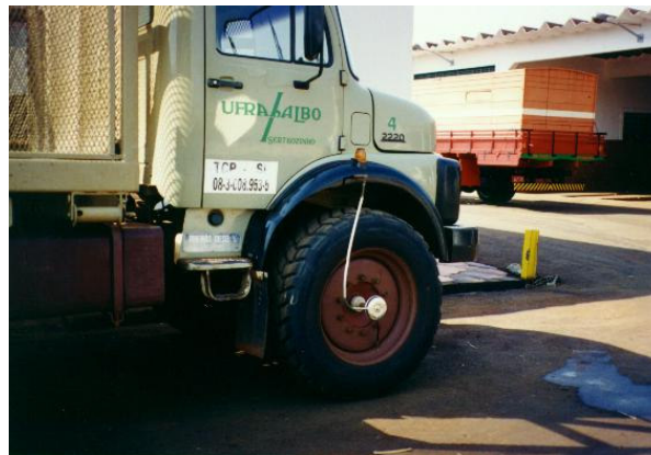
Figure 4. Trelleborg tire in a steering single (40 cm wide).
