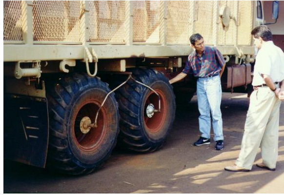
Figure 5. Trelleborg tire in a tandem axle (60 cm wide).
