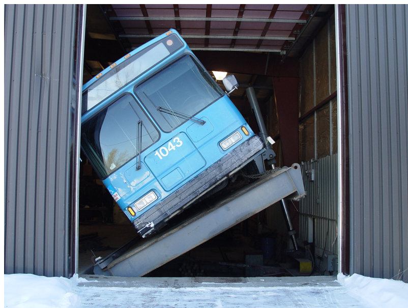
Figure 11 - Series drive hybrid bus on tilt table
