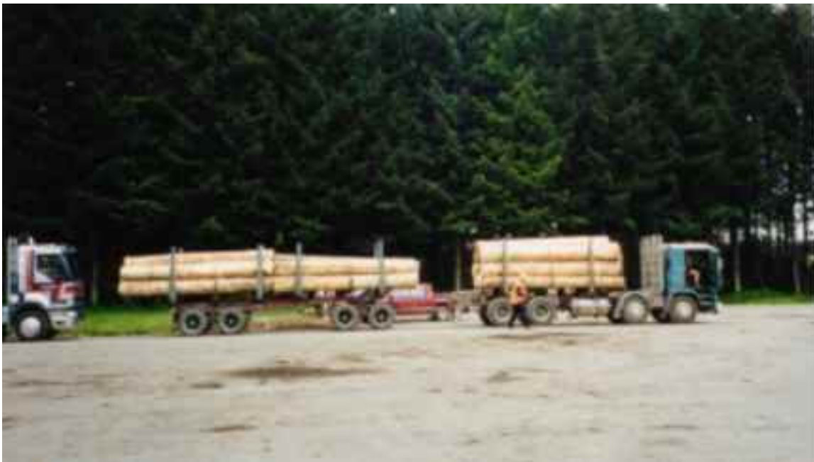
Figure 6. 22m multi-bolster log load compared to 20m single bolser load.
