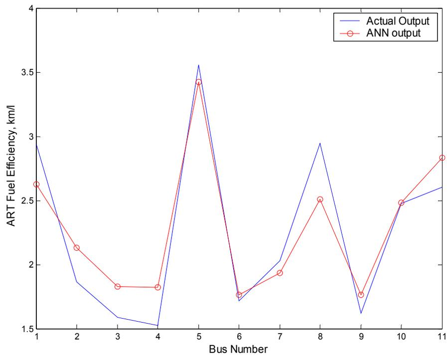
**Figure 7. Comparison plot for ART fuel efficiency on test set.**
