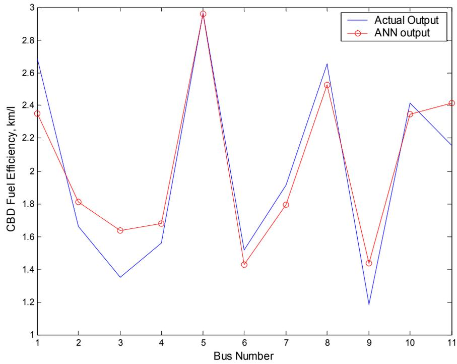
**Figure 6. Comparison plot for CBD fuel efficiency on test set.**
