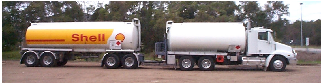
Figure 1. Original truck trailer design -19 meters (62 feet), 50 tonnes (110,000 pounds)
