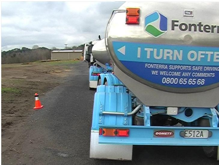
**Figure 5. Full truck and empty trailer with EBS/NZHVBC brake system from 50 km/h.**
