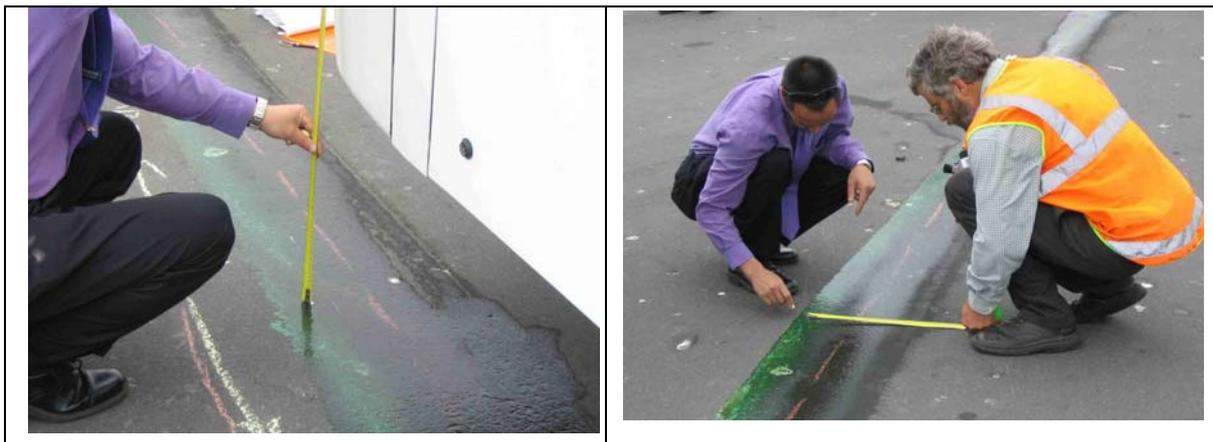
**Figure 2. Tail swing measurement.**
