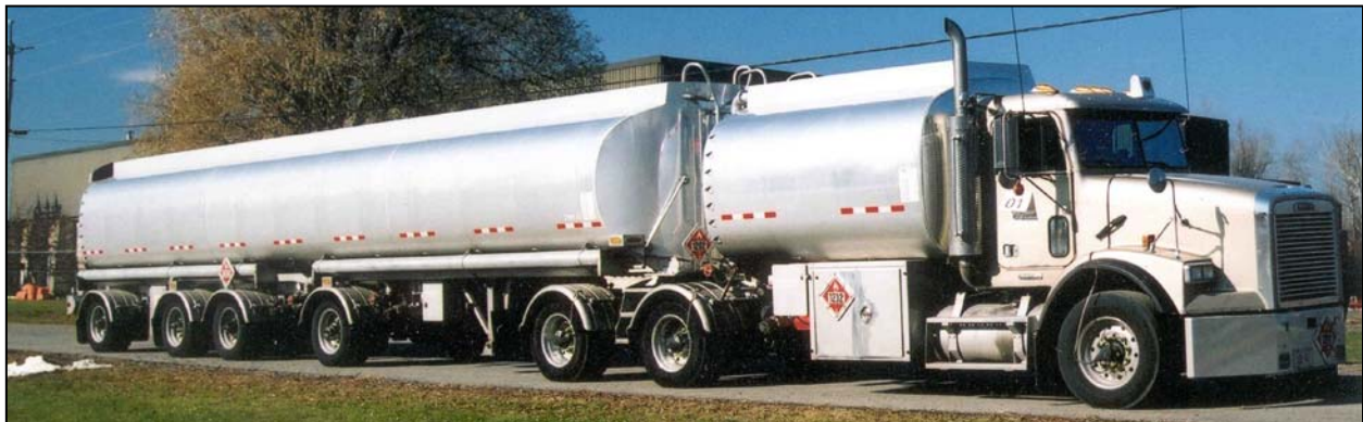
Figure 2: Vehicle 01, 7-axle Tractor-semitrailer with Drome Tank on Tractor
