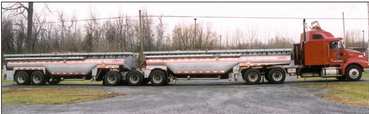
Figure 3: Vehicle 02, 8-axle Low-profile B-train
