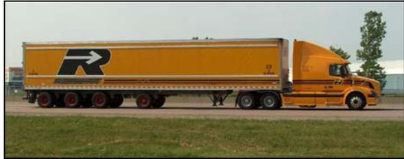
**Figure 6** – Self-steer Quad Semitrailer
