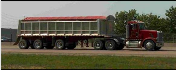
**Figure 5** – Self-steer Triaxle Semitrailer
