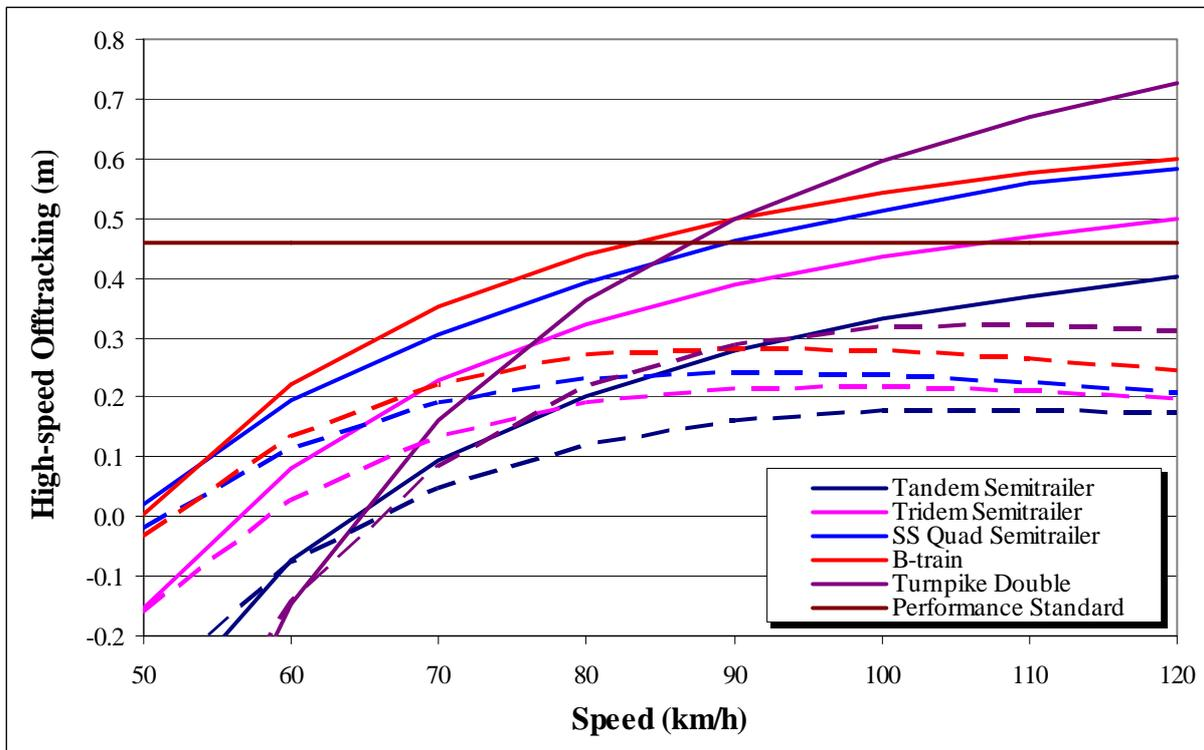
**Figure 11 – High-speed Offtracking for Various Configurations**
