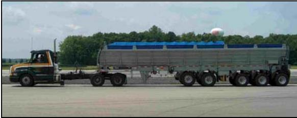
**Figure 7** – 5-axle 113 Semitrailer
