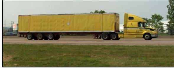
**Figure 4** – Tridem Semitrailer
