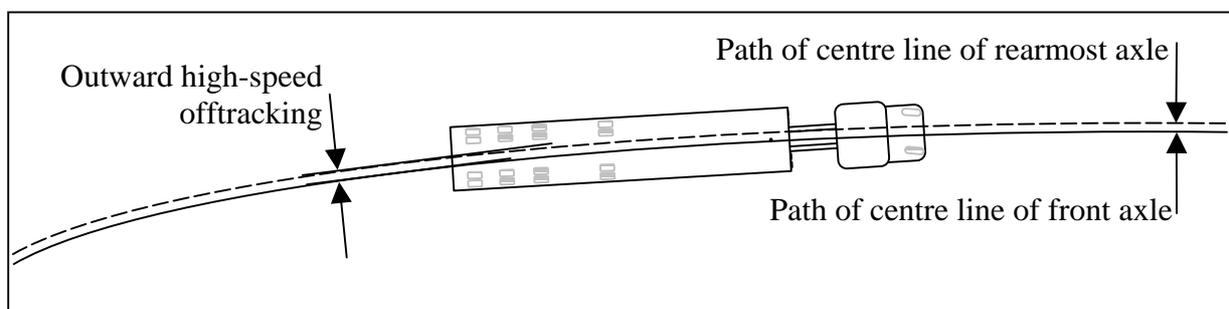
**Figure 1** – High-speed Offtracking in a High-speed Turn
