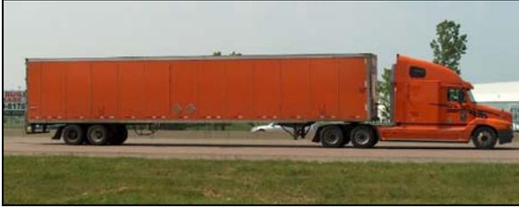
**Figure 3** – Tandem Semitrailer
