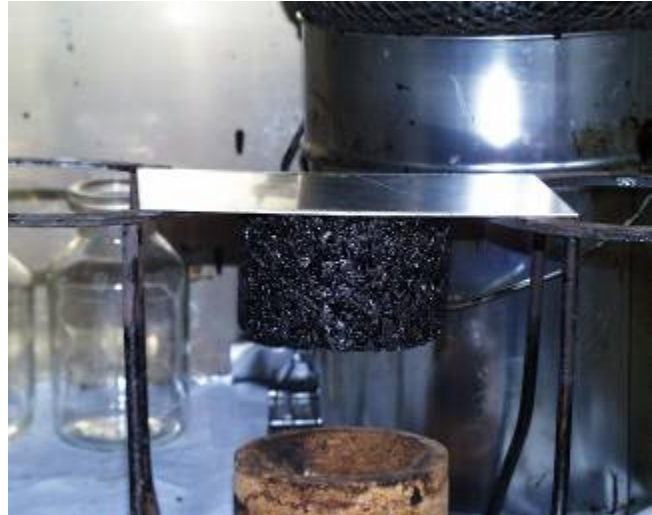
Figure 5 – Marshall specimen glued on an alloy plate in the oven.
