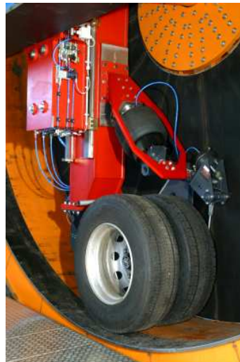
Figure 11 – Truck wheel station at PFF with twin tyre assembly
