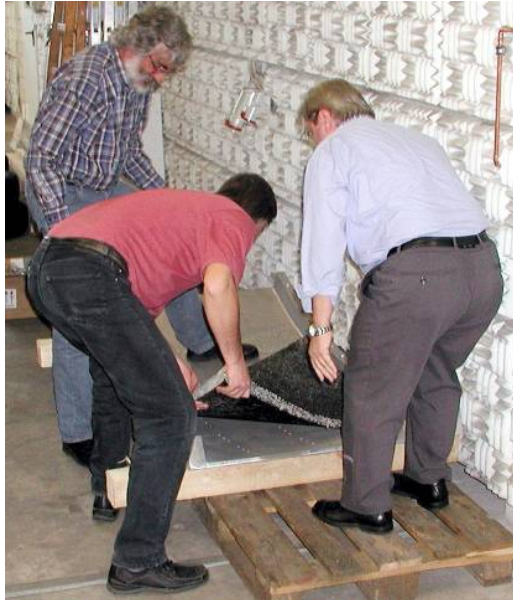
Figure 4 – Bending of a road surface slab into the casket shape.
