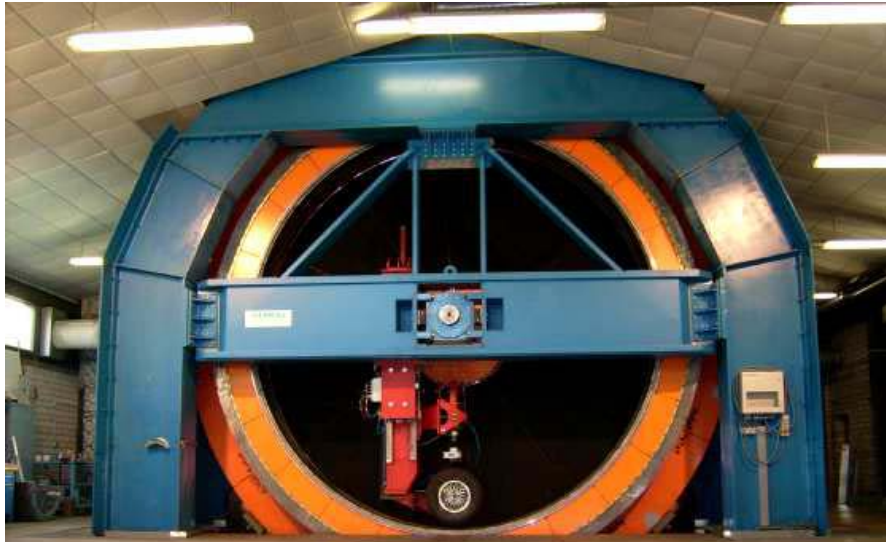
Figure 1 – The Tyre Road Interaction Test Facility (PFF) of BAST.
