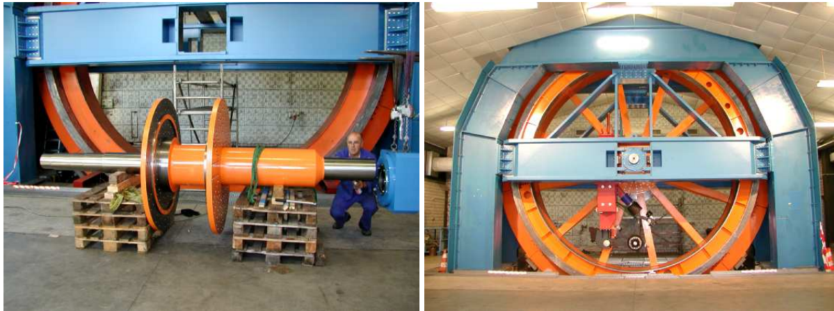
Figure 2 – Reconstruction of the PFF: traverse shaft spokes (uncovered).
