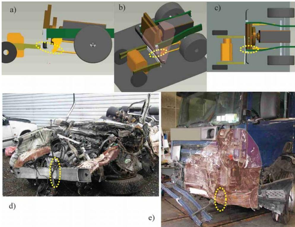
**Figure 4** – Case I. 3D geometric models of the vehicles at the position just before the accident: a) side view, b) isometric view, c) top view. The vehicles after the accident: d) the car, and e), f) the truck. The dashed ellipses indicate matching impact points.
