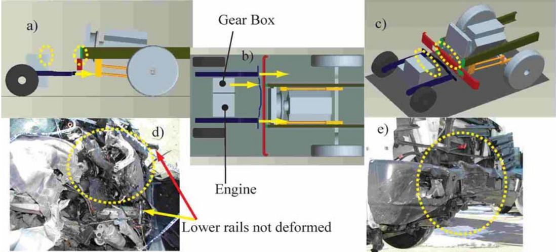
**Figure 8** – Case IV. 3D geometric models of the vehicles at the position just before the accident: a) side view, b) top view c) isometric view. The vehicles after the accident: d) the car and e) the truck. The dashed ellipses indicate the matching impact points.
