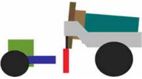
Figure 9 – Solution proposed for making use of truck cooler as energy absorbing element during an accident
