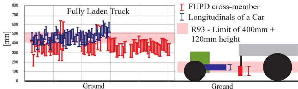
**Figure 1** – Comparison between position of FUP cross-members when trucks are fully laden, and longitudinals of cars. A limit for FUP cross-member clearance and its section height in accordance with Regulation 93 is included.
