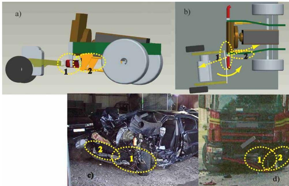
**Figure 5** – Case II. 3D geometric models of the vehicles at the position just before the accident: a) side view, b) top view. The vehicles after the accident: c) the car and d) the truck. The dashed ellipses indicate the matching impact points before and after car rotation.
