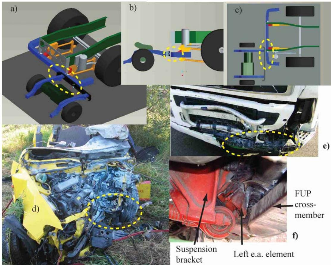
**Figure 6** – Case III. 3D geometric models of the vehicles at the position just before the accident: a) isometric view, b) side view c) top view. Photos of the vehicles after the accident: d) the car and e) the truck, and f) deformed left e. a. element. The dashed ellipses indicate the matching impact point.
