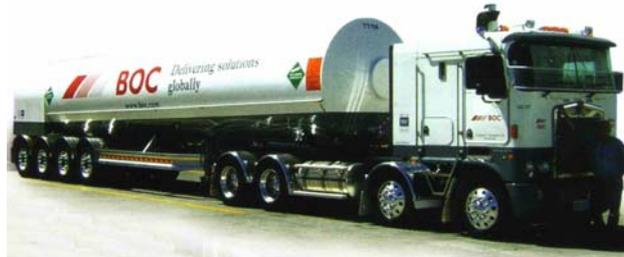
**Figure 1** – Example CO<sub>2</sub> road tanker
