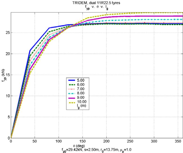
Figure 4 – Peak scuffing force against angle of turn for different wheelbases.
