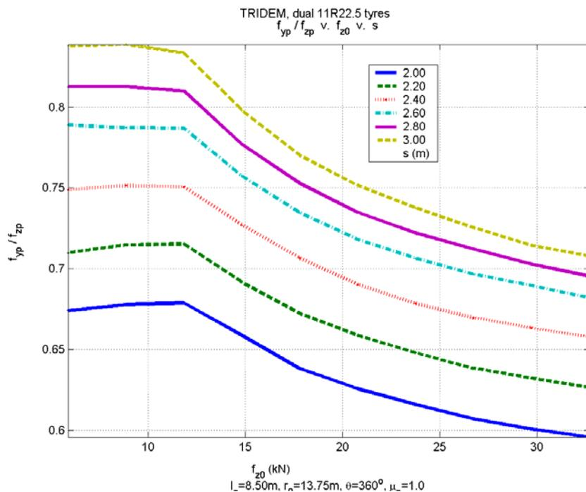
**Figure 3 – Ratio of peak scuffing force to peak vertical force against static load.**
