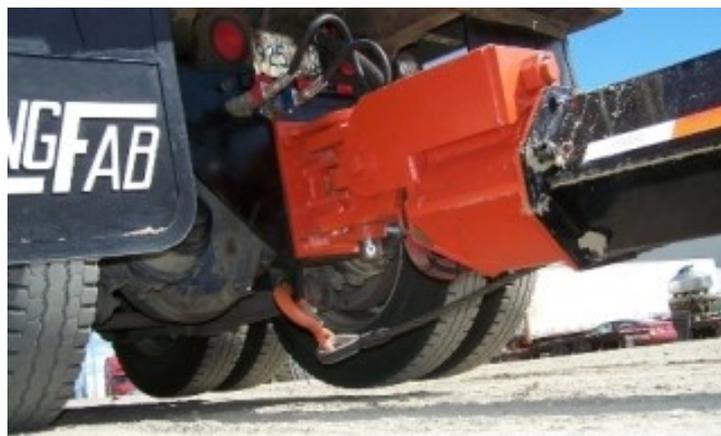
**Figure 3. Wolf Trailers roll-coupled pony-trailer hitch**
