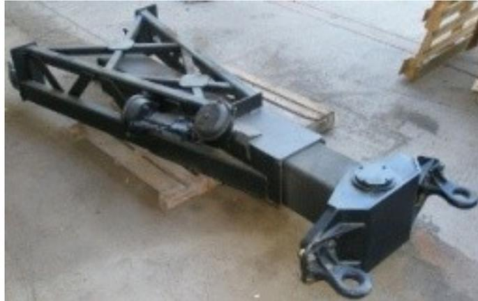
**Figure 2. Feric prototype full-trailer drawbar**
