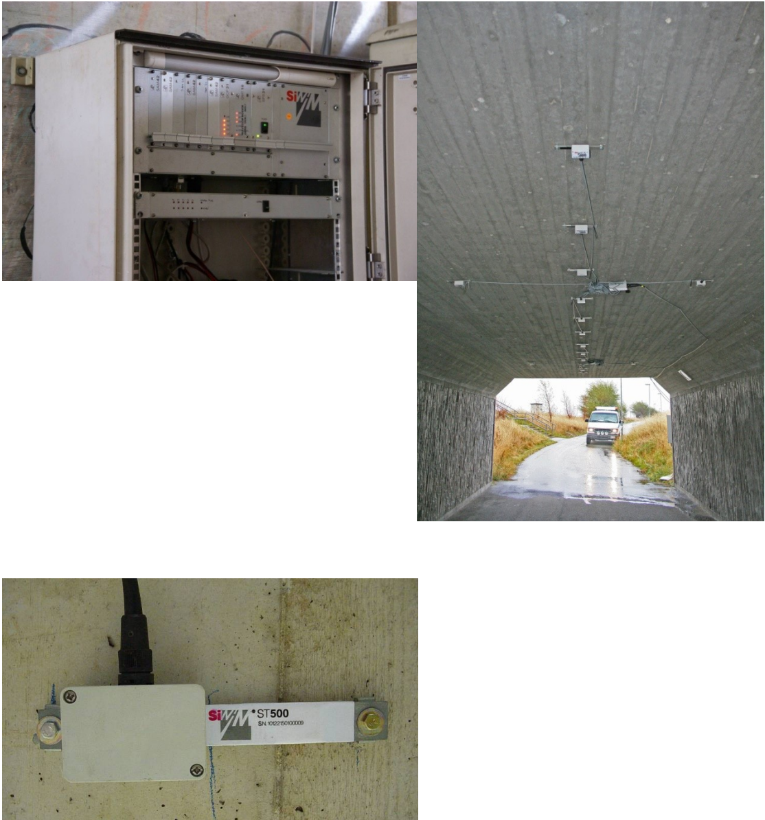
Figure 1 - Left -The system installed at a site in southern Sweden, Top right – The signal processing unit, Bottom right – Strain transducer
