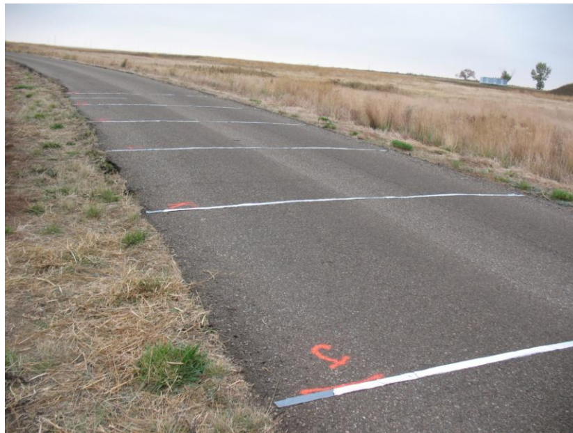
Figure 6. Tape on test track for measuring off-tracking
