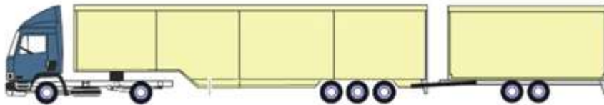
Type 2: Tractor-Semitrailer and Center Axle Trailer, max. length 25,25 m
