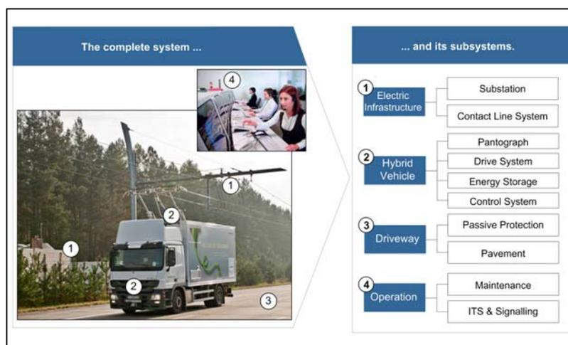
**Figure 2 – The eHighway system and its sub-systems**
