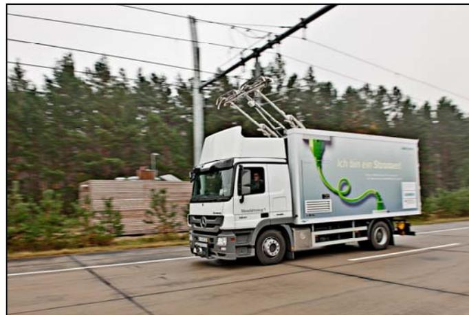
**Figure 6 – Vehicle with current collector**
