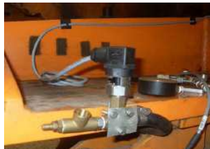
Figure 4- Air pressure transducer (APT)
