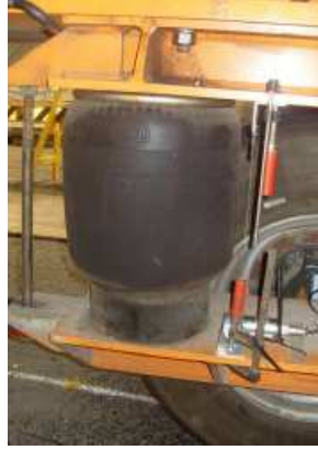
Figure 3- Air cushions suspension similar to HDV
