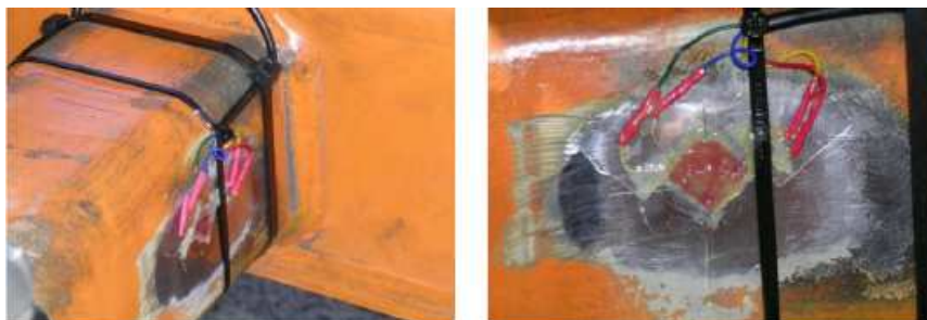
Figure 6- Strain gauges on wheel axle
