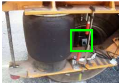
Figure 5- Accelerometers on wheel hub
