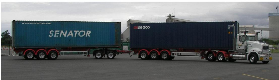
**Fig. 3 - PBS approved Haulmark Steering A-Double**
