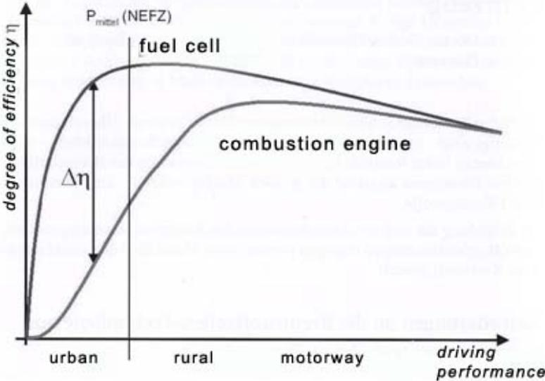
**Figure 1 - Efficiency of combustion engine and fuel cell (Docter et al. 2006)**
