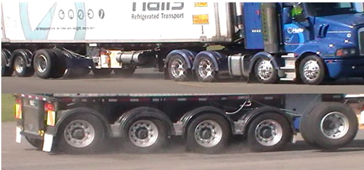
**Figure 6: Steer angle on axles 3 and 4, UWC – 105 m radius – 64 km/h – 26 tonne**
