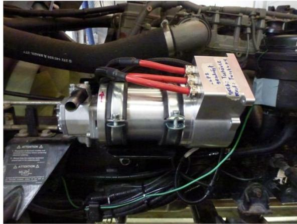
**Figure 11 – Synchronous motor and hydraulic pump for EHPS system built-in in a CV**
