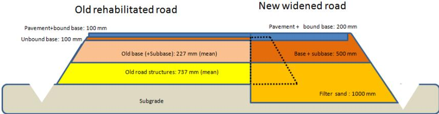
**Figure 5 – The principles of the proposed third lane structure**
