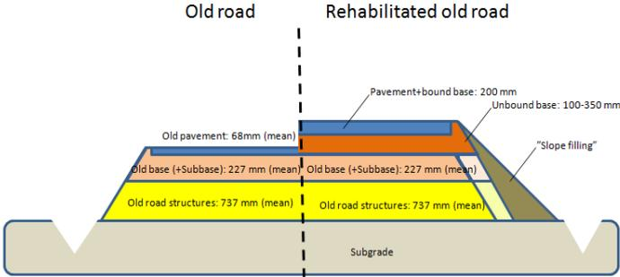
**Figure 4 – The principles of the proposed basic structure for strengthening**
