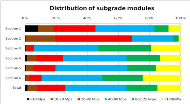
**Figure 1 – The distribution of subgrade moduli**
