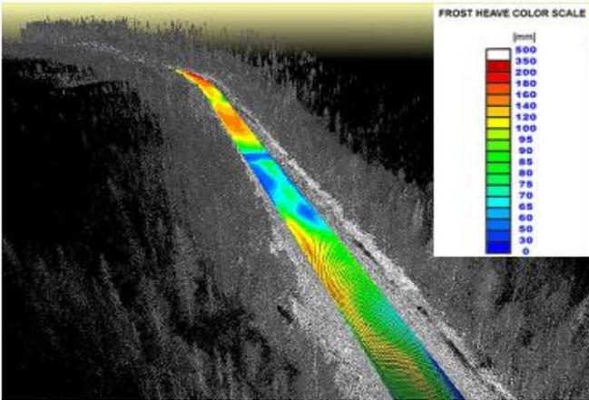
Figure 2 – An example of frost heave point cloud data
