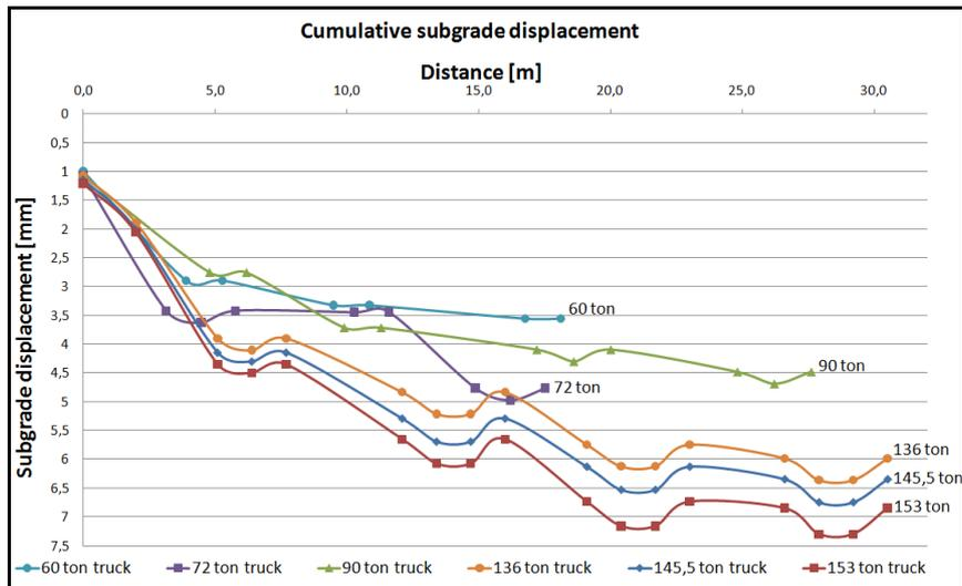
**Figure 7 – The cumulative displacement of weak subgrade (modulus 10 MPa) calculated for each truck option**
