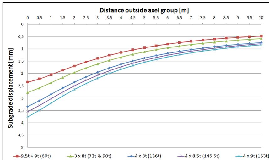
**Figure 6 – Comparison of the truck options on weak subgrade (modulus 10 MPa) based on the heaviest axle group of each option**
