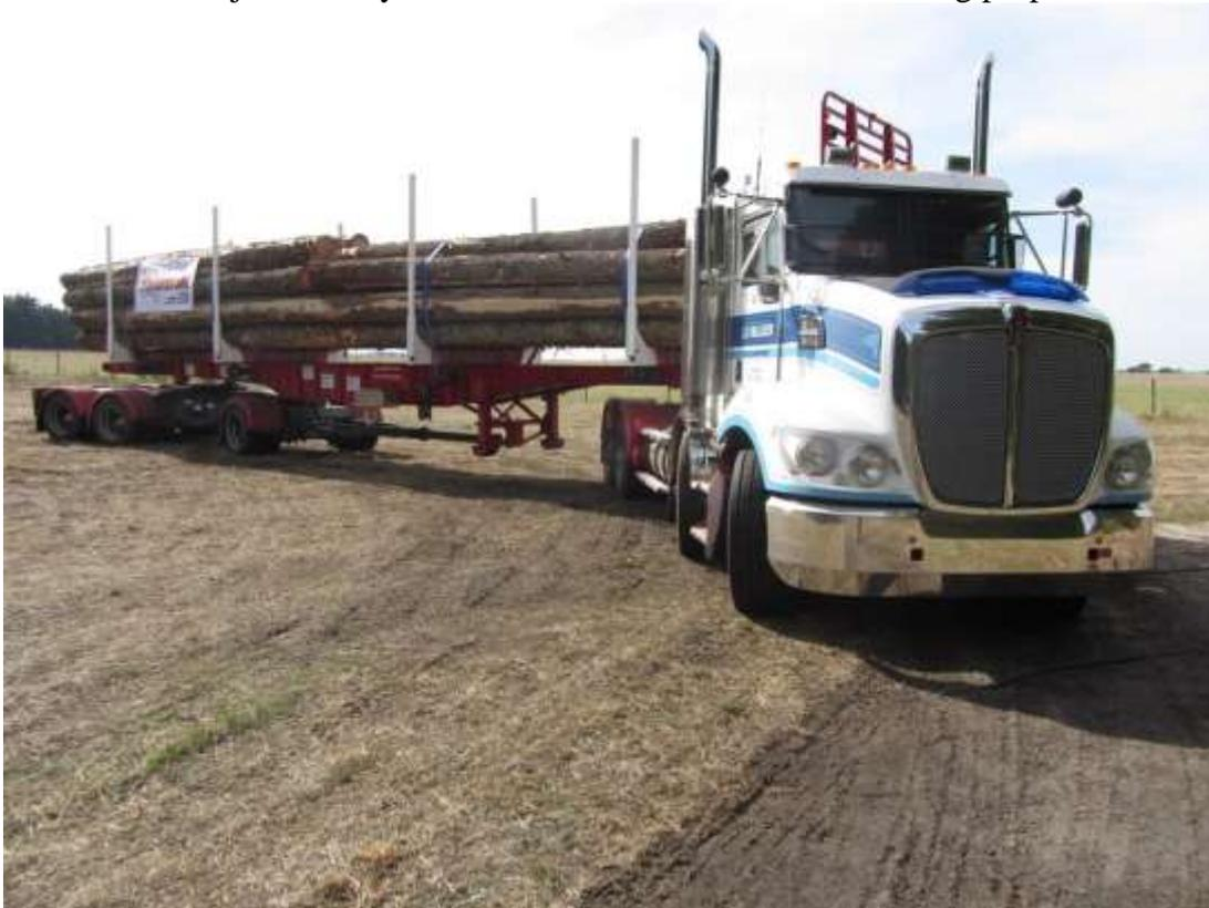
**Figure 3. Prototype Easysteer trailer configured for log transport.**
