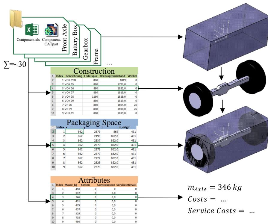
Figure 7: Structure of database with Excel tables and CATIA part
