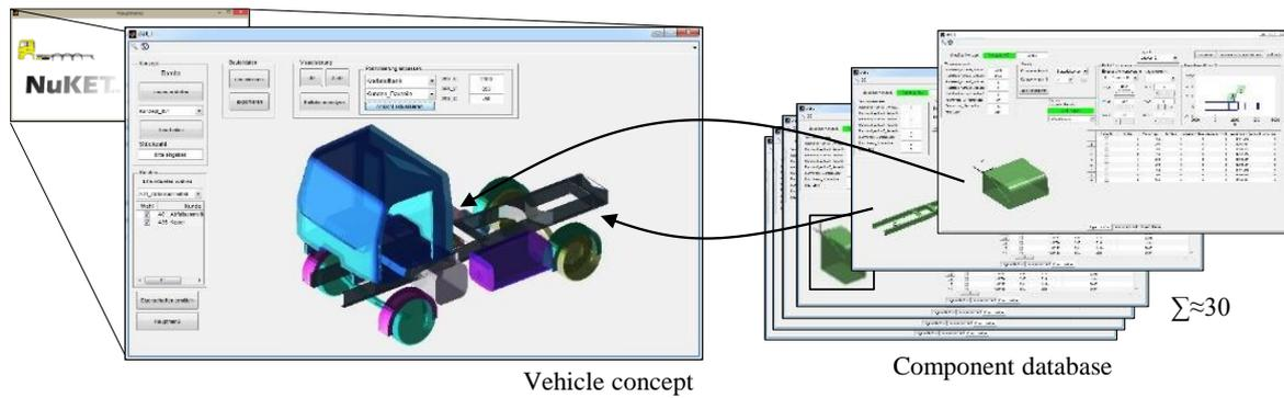
Figure 3: Development of vehicle concept based on abstracted component geometry and basic characteristics [cf. 5]
