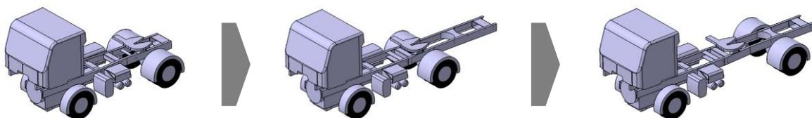
Figure 9: Exemplary vehicle concept manipulation (frame variant and wheel base)
