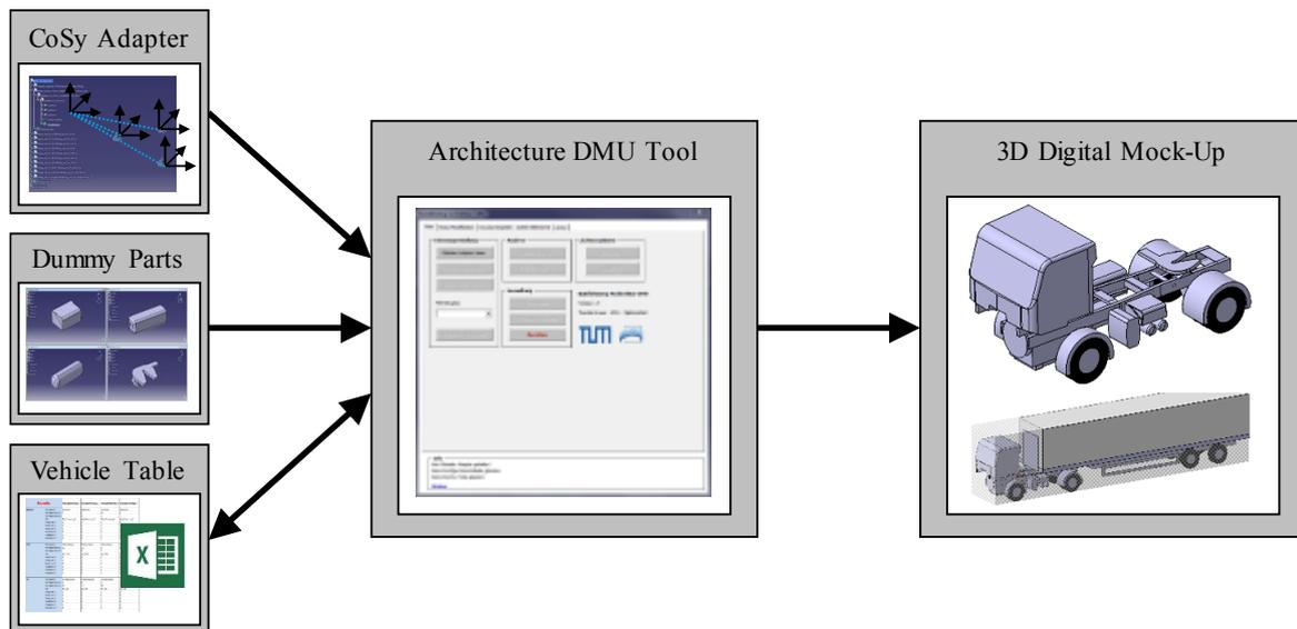
Figure 8: Tool structure of the Architecture Digital Mock-up (A-DMU)
