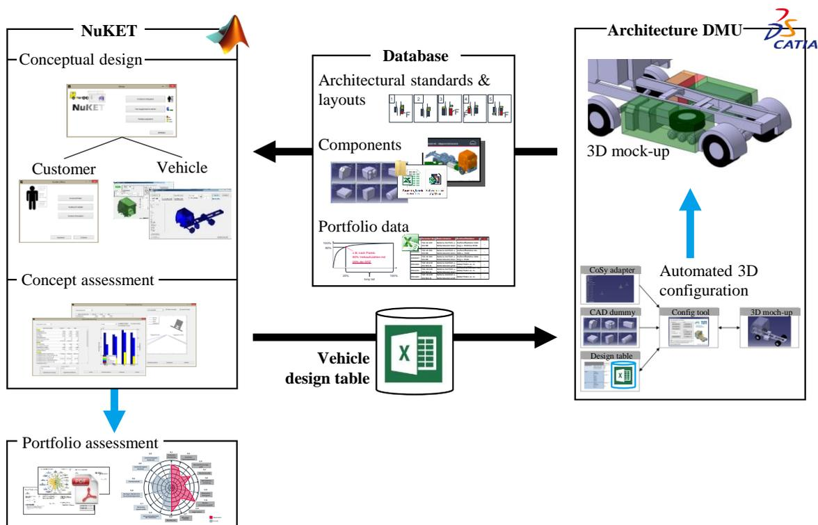
Figure 1: Integrated tool chain for commercial vehicle concept design and assessment [cf. 5]
