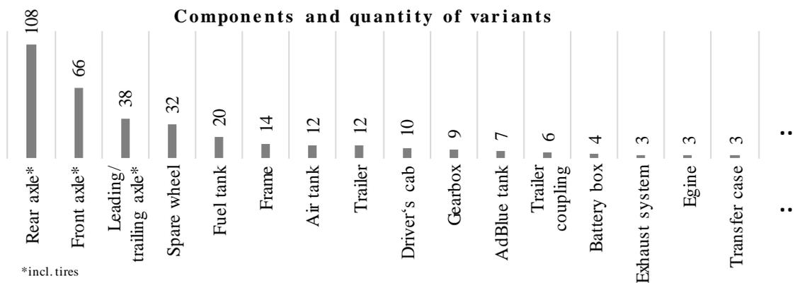
Figure 6: Included components and quantity thereof
