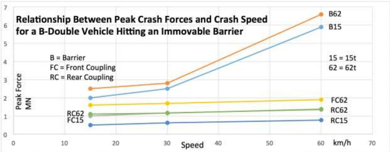
**Figure 7** Peak force for both masses plotted against initial speed; for the B-double truck.
