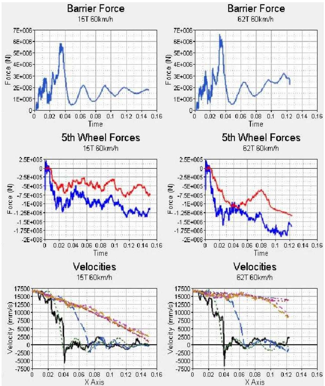
**Figure 8c** Force and velocity results for 60 km/h impacts.
