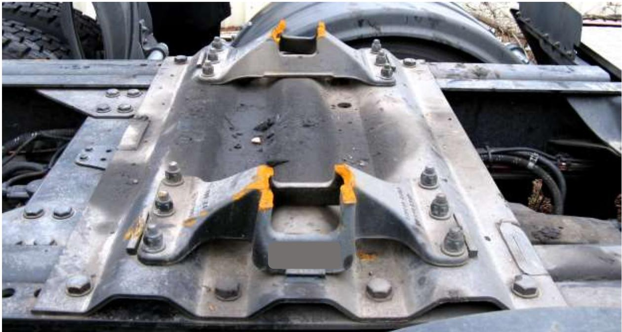
**Figure 1** Failed fifth wheel (cast) pedestal legs on a fifth wheel fitted to a truck-tractor.
