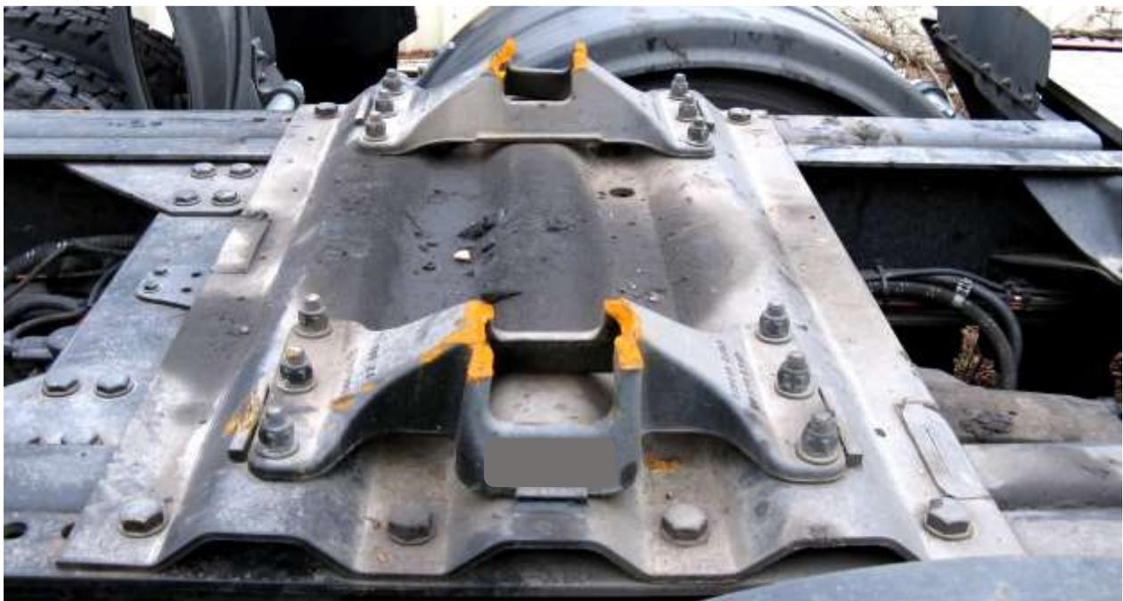
**Figure 1** Failed fifth wheel (cast) pedestal legs on a fifth wheel fitted to a truck-tractor.
