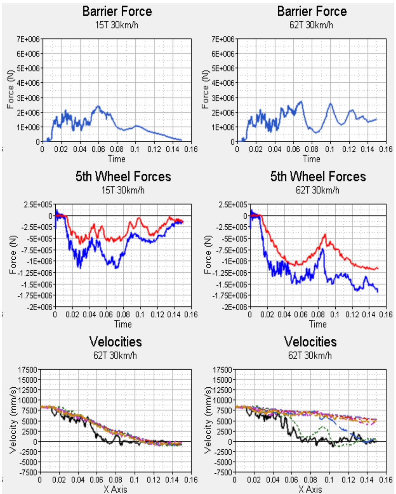
**Figure 8b** Force and velocity results for 30 km/h impacts.
