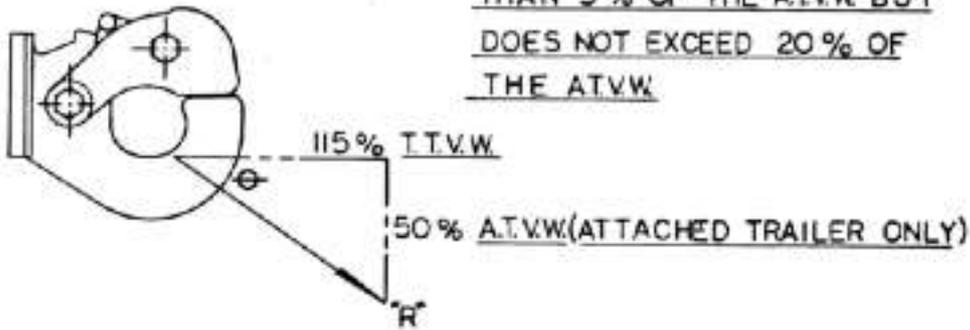
**Figure 10** The proof-test specification that is in SAE J847.
