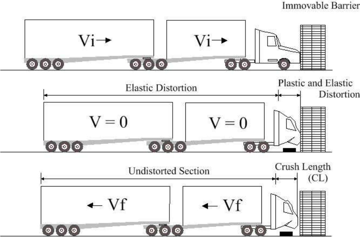
**Figure 3** Simplistic representation of plastic and elastic sections of the crash vehicle.
