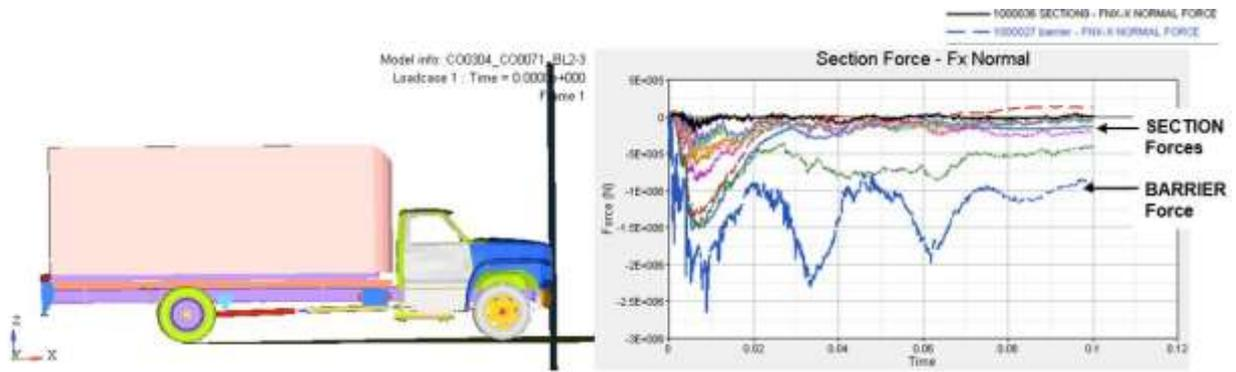
**Figure 3a** Force results for the barrier crash
