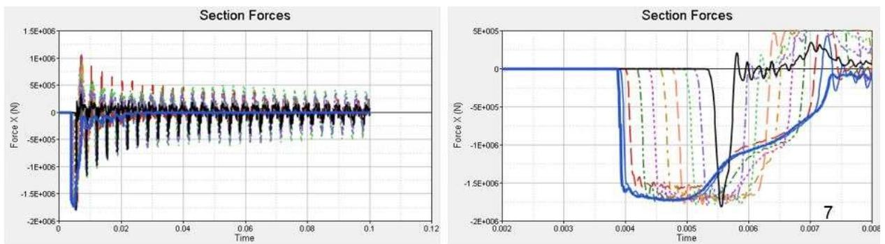
**Figure 4** Shock waves in the chassis-rail ladder of the rigid truck
