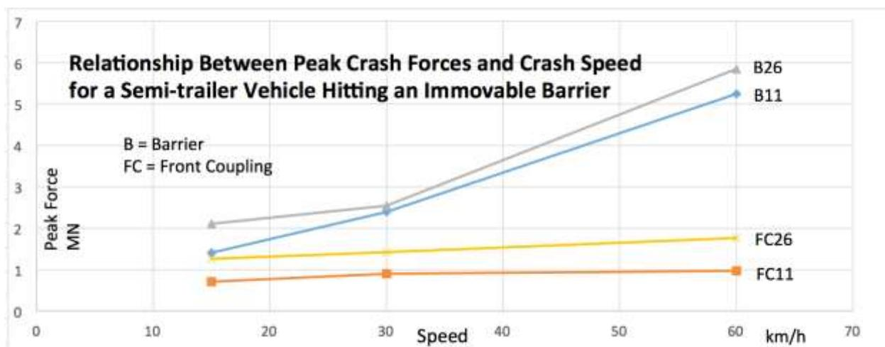
**Figure 9** Peak force for both masses plotted against initial speed; for the B-double truck.
