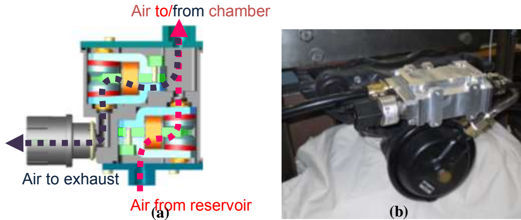
Figure 4 - CVDC valve manifold for individual wheel braking control. CAD model (left), prototype valve block positioned next to brake chamber (right)
