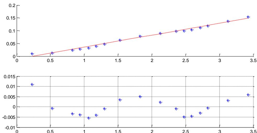
**Figure 4 –Top: height of the individual laser tracks (blue) and the derived crossfall (red) for one sample. Bottom: the height of the laser tracks after the crossfall has been subtracted.**
