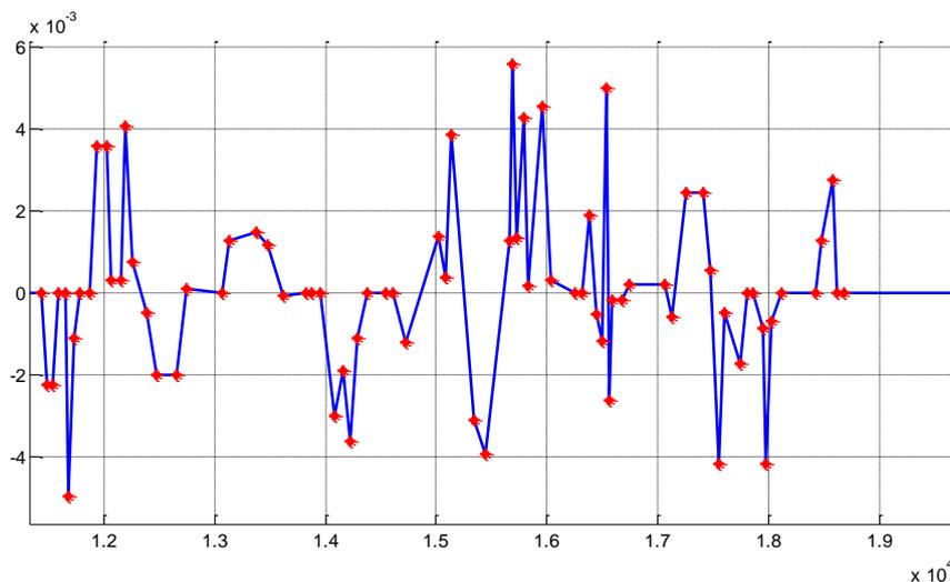
**Figure 3 – Road curvature (1/m) as a function of distance (m) for part of the road**
