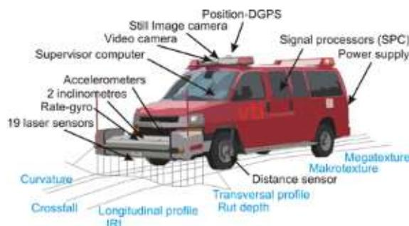
**Figure 1 - VTI Road Surface Tester (RST)**
