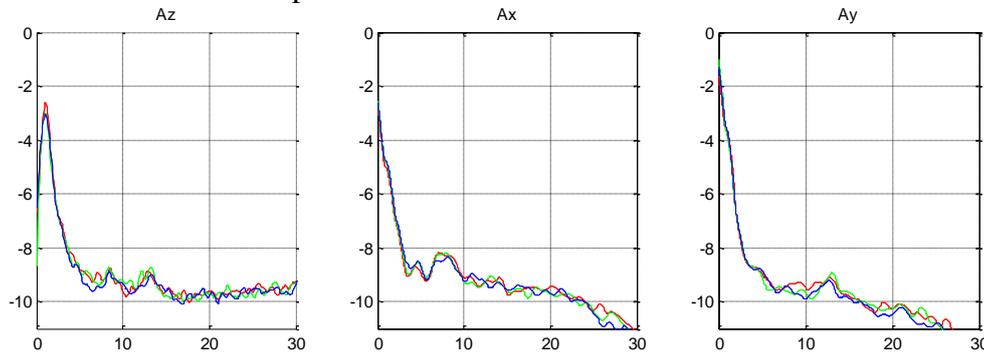
**Figure 8 – PSD energy content plotted in log scale as a function of frequency for vertical (Az), longitudinal (Ax) and lateral (Ay) accelerations for three separate measurements.**
