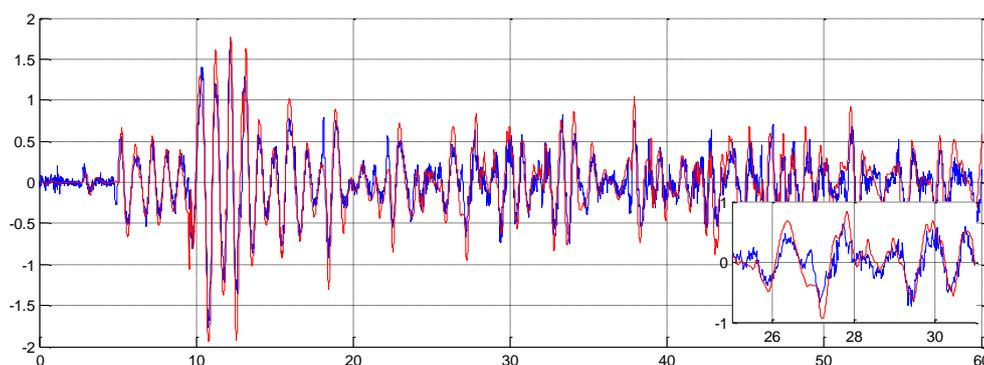
**Figure 7 – Vertical acceleration ( $\text{m/s}^2$ ) plotted as a function of time. Measured (blue) and simulated (red). Closeup in the right corner.**
