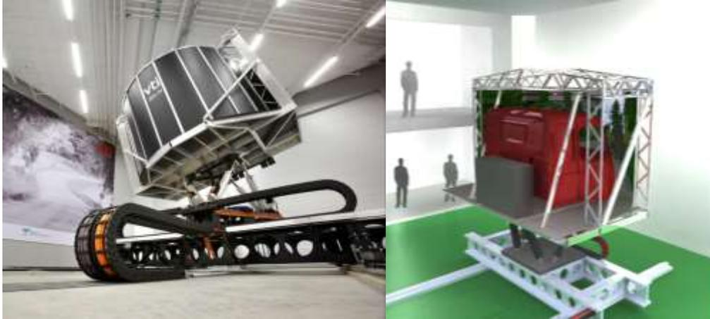
**Figure 5 - The VTI Sim IV moving base driving simulator**
