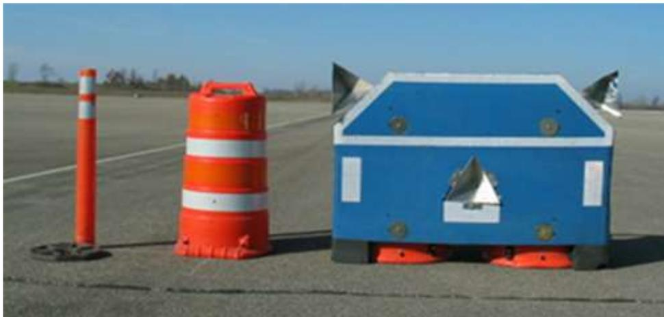
**Figure 2. Final UMTRI fixed vehicle targets compatible with radar and vision systems**
