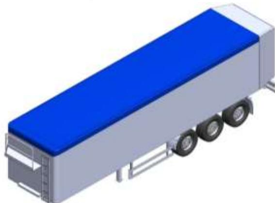
**Figure 5 – Drawing of a streamlined semi trailer, the boat tail can be seen at the rear of the semi trailer**
