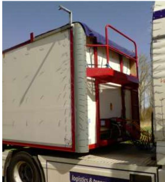
**Figure 4 – a rounded leading edge on the test vehicle**
