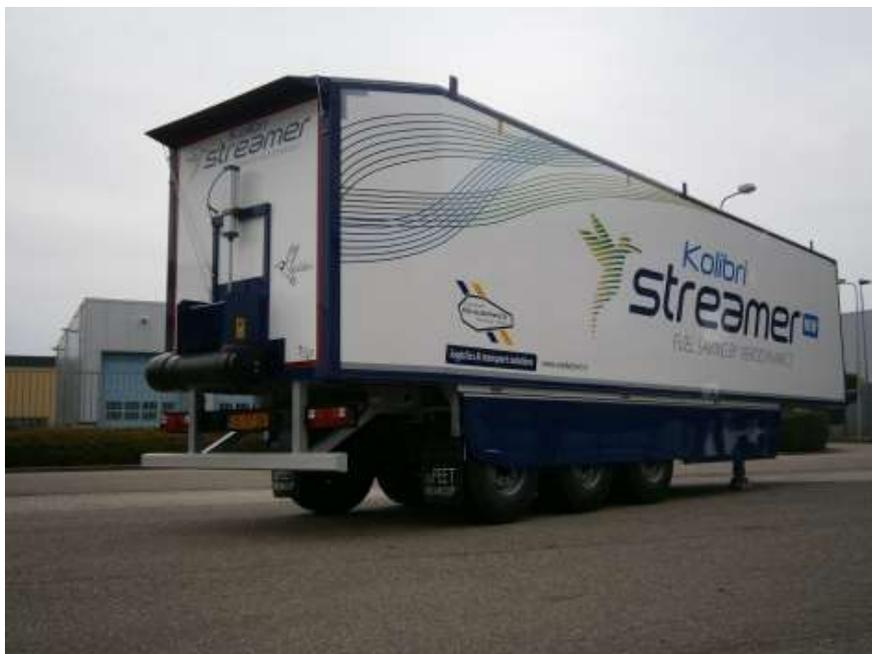
**Figure 9 – The production version of the aerodynamic semi trailer, the Kolibri Streamer.**
