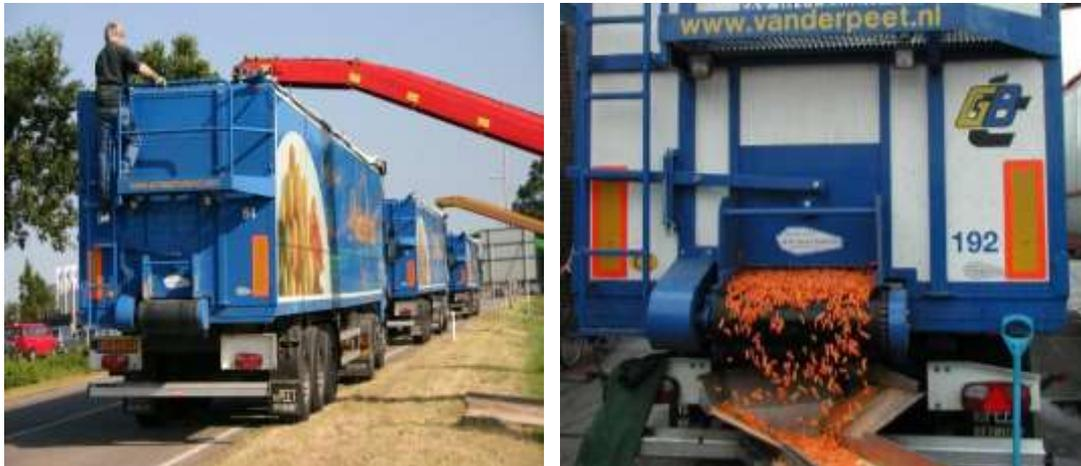
**Figure 1 – The standard Kolibri semi trailer loading (left) and unloading (right)**
