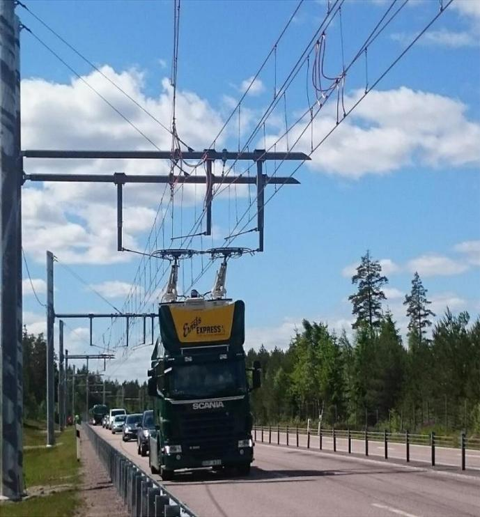
**Figure 3 - The Siemens e-Highway system demonstrated outside Sandviken in Sweden.**
