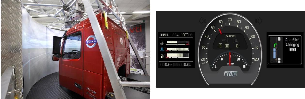
Figure 2: On the left, truck cab mounted on SimIV. On the right, developed HMI including feedback of the traffic situation management functionality.
