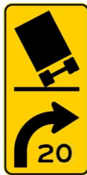
Figure 9 Australian Advisory Curve Speed Sign for Heavy Vehicles
