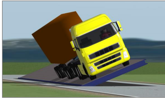
Figure 6 TruckSim® Model of a Vehicle Combination on Tilt Table
