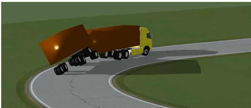
Figure 8 The Trailer Overturned at 49 km/h in the Entry Ramp
