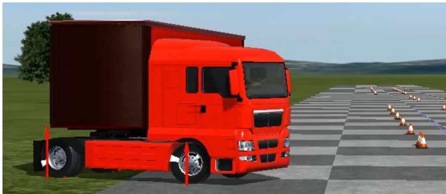
Figure 2 – Semitrailer Rig Jackknifes on Approved Winter Road Slipperiness; \mu = 0.25
