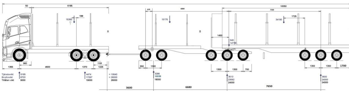
**Figure 8: ETT:2 combination dimensions**
