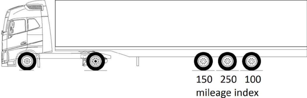
**Figure 13 Tire wear on semitrailer triple**
