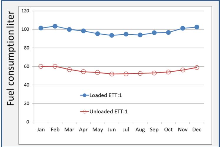
**Figure 11 Average fuel consumption per month taken as average from January 2009 until September 2014 for the first combination ETT:1. The fuel consumption is more than 10% lower during the summer compared to winter.**
