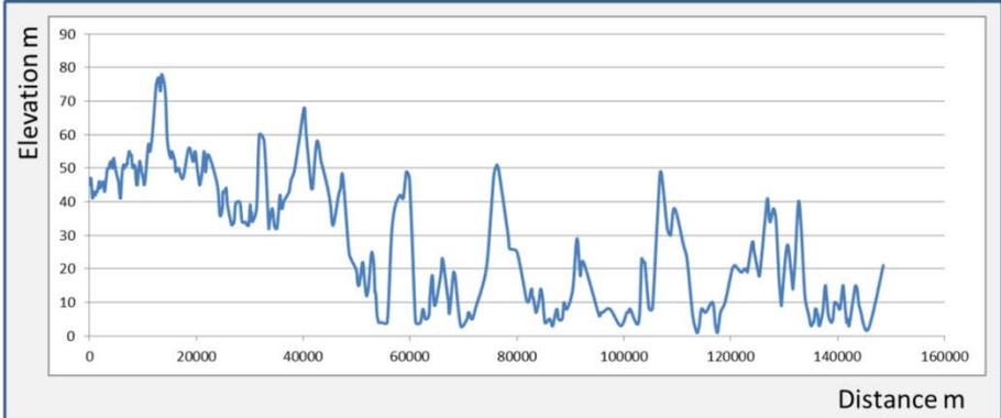
**Figure 4 Elevation curve for transport seen from Överkalix to Piteå. Maximum elevation is 80 meter and minimum is almost at sea level.**
