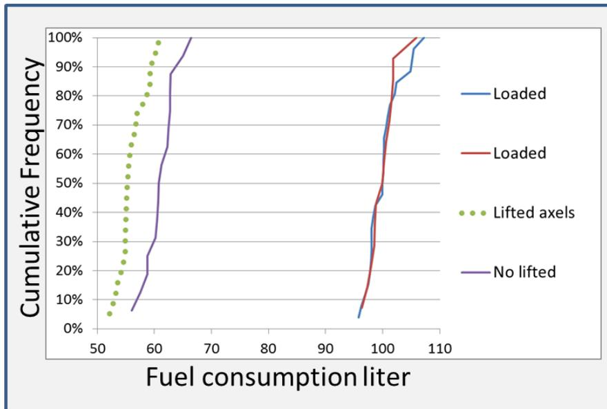
**Figure 15 Cumulative frequency of fuel consumption for impact of axle lifting on return trips. The loaded curve shows comparable conditions for the test. The difference on the unloaded return trip is only dependent on the five lifted axels.**
