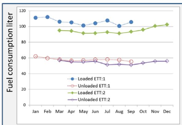
**Figure 10 Fuel consumption during 2014. The ETT:2 shows an overall fuel consumption that is 9% lower than ETT:1.**
