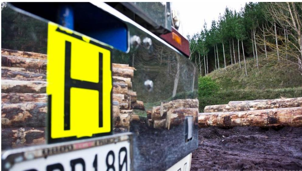
**Figure 2: All HPMVs are required to clearly display their H plate front and rear**
