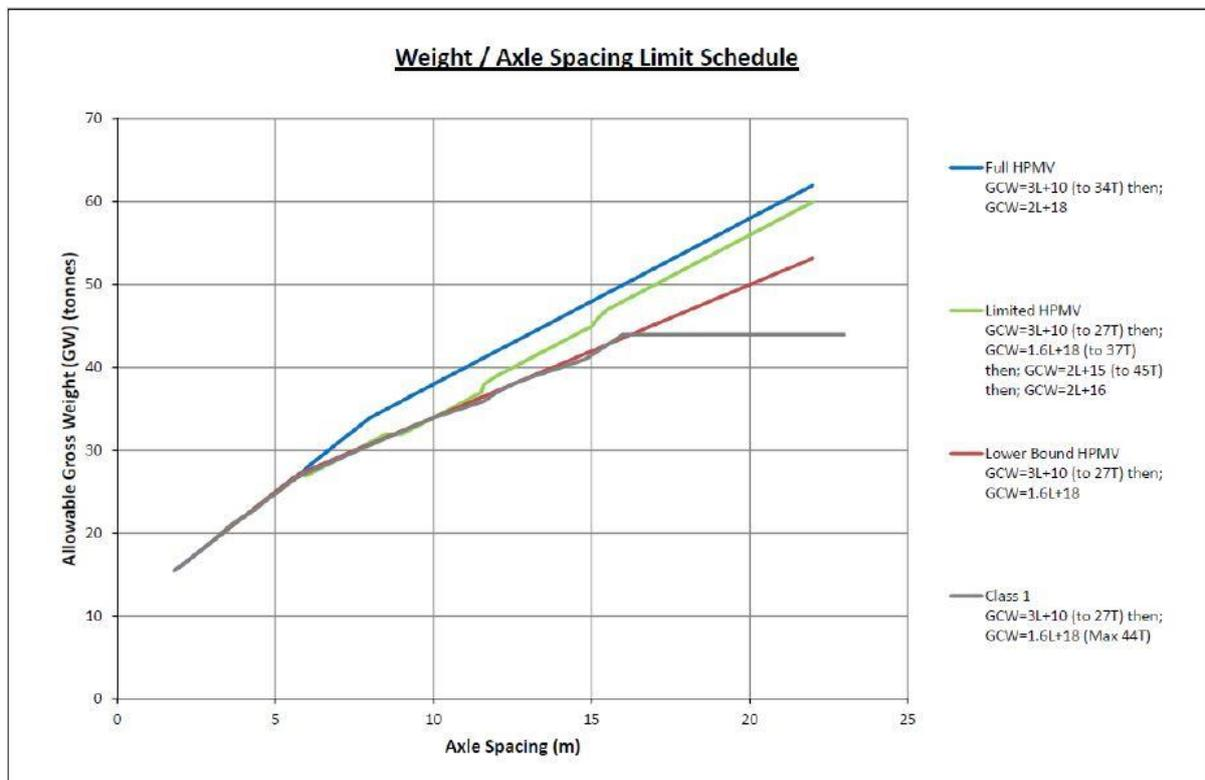
**Figure 1: Allowable Gross Weight vs Axle Spacing for Full, Limited and Lower Bound (50MAX) HPMVs**
