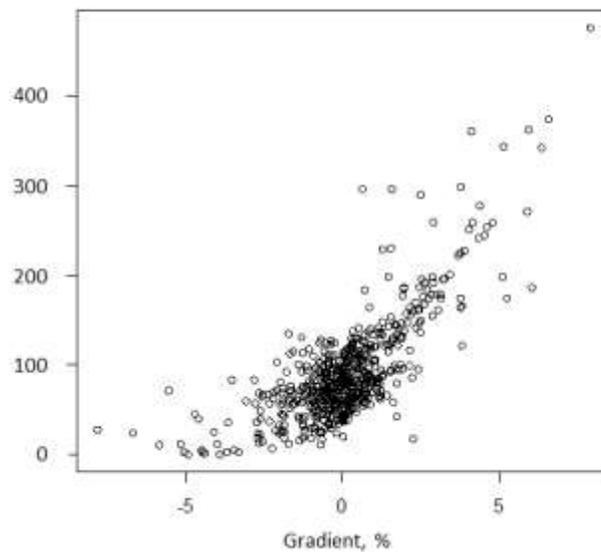
**Figure 4 – A scatter plot of fuel consumption (litres/100 km) and road gradient (%).**
