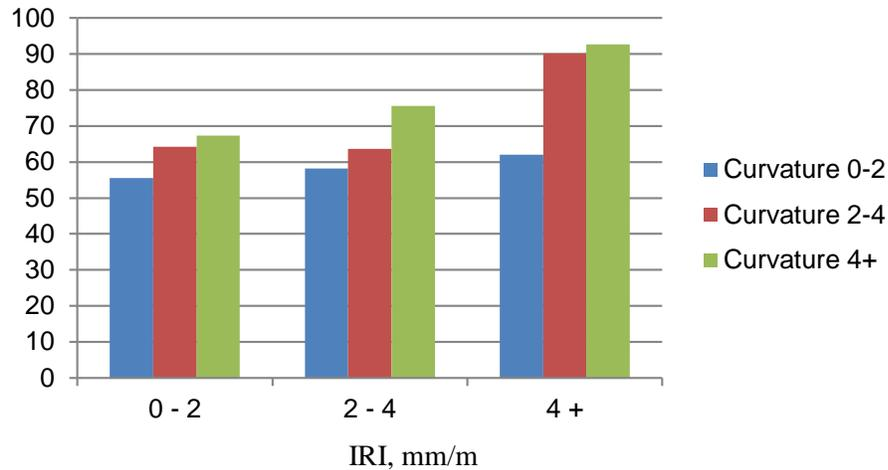
**Figure 3 – Average fuel consumption (litres/100 km) for different classes of road surface roughness (mm/m) and curvature (1000/r).**
