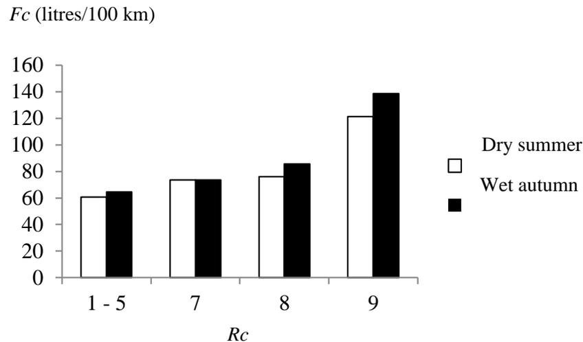
**Figure 2 – Average fuel consumption (litres/100 km) per functional road class (Rc) for the dry summer and wet autumn replication.**
