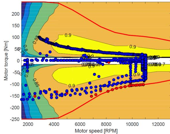
**Figure 7 – Optimized motor operating points during CO<sub>2</sub> cycle**
