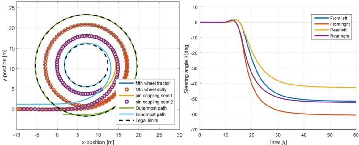
**Figure 4 – A-double trajectory (left) and dolly steering angles (right) during simulation of a 360-degree turn**
