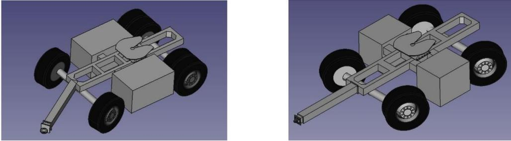
**Figure 2 – 4x2 dolly design with mechanical linkage steering (left) and 4x4 dolly design with four wheel steering (right) to be used in the A-double HCV**
