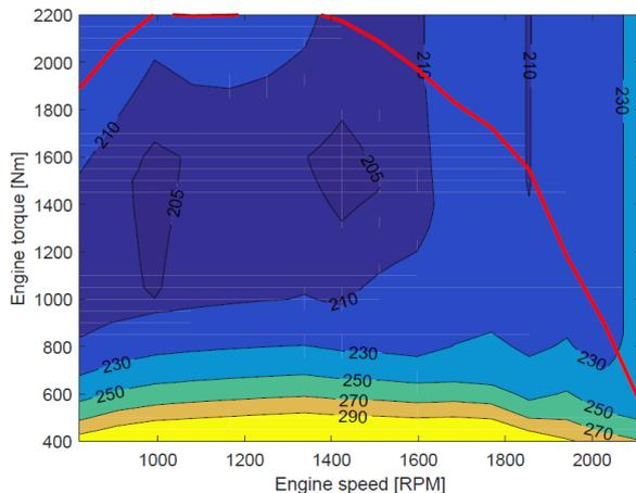
**Figure 6- Generic EURO-6 fuel map, showing BSFC in [g/kWh]**
