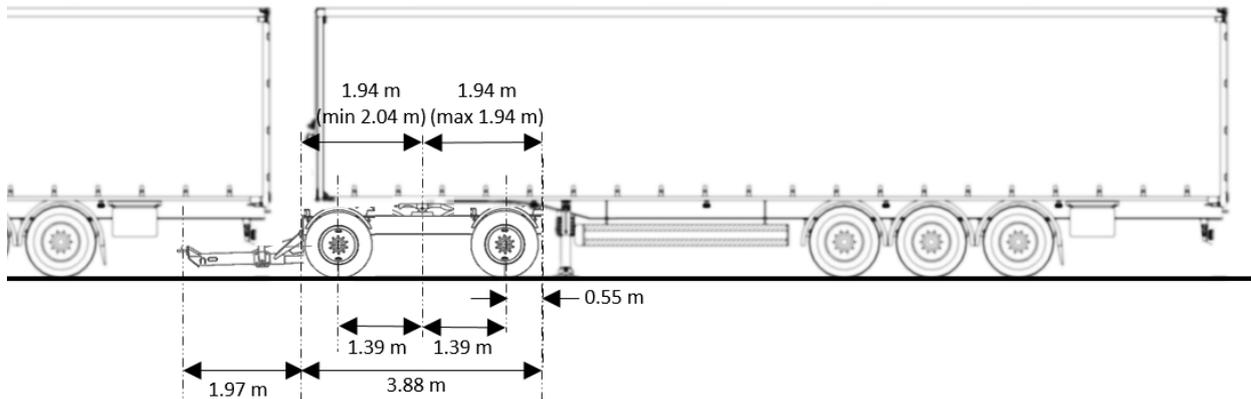
**Figure 3 – Final dimensions and locations of the 4x4 dolly design in the A-double HCV**
