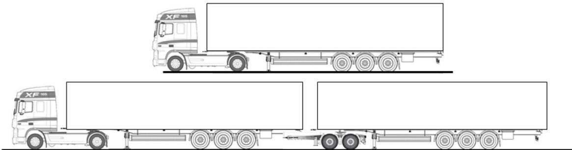
**Figure 1 – EU tractor semi-trailer combination (top) and A-double HCV (bottom)**
