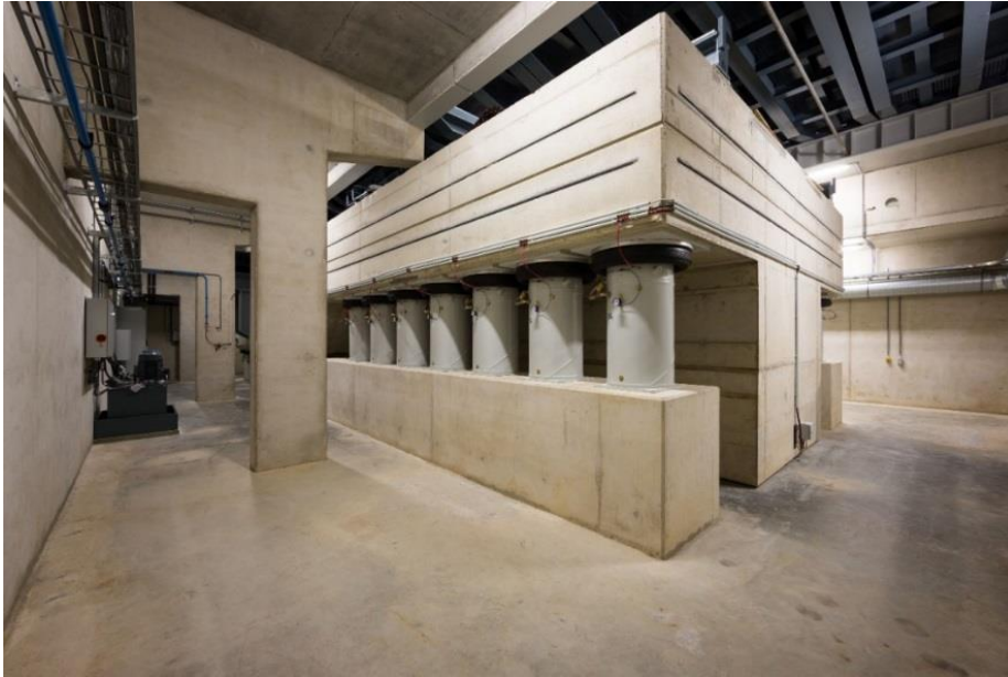
Figure 3.: The suspended test bench support (32 air bellows)
