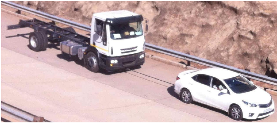
Figure 3: A test vehicle (Iveco Eurocargo 120e21 truck) is towed at constant velocity, while the front brake pressure is applied to the test vehicle
