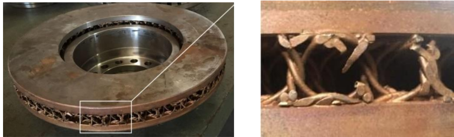
Figure 2: Custom made brake disc with Wire-woven bulk diamond (WBD) core used in the ventilated channel
