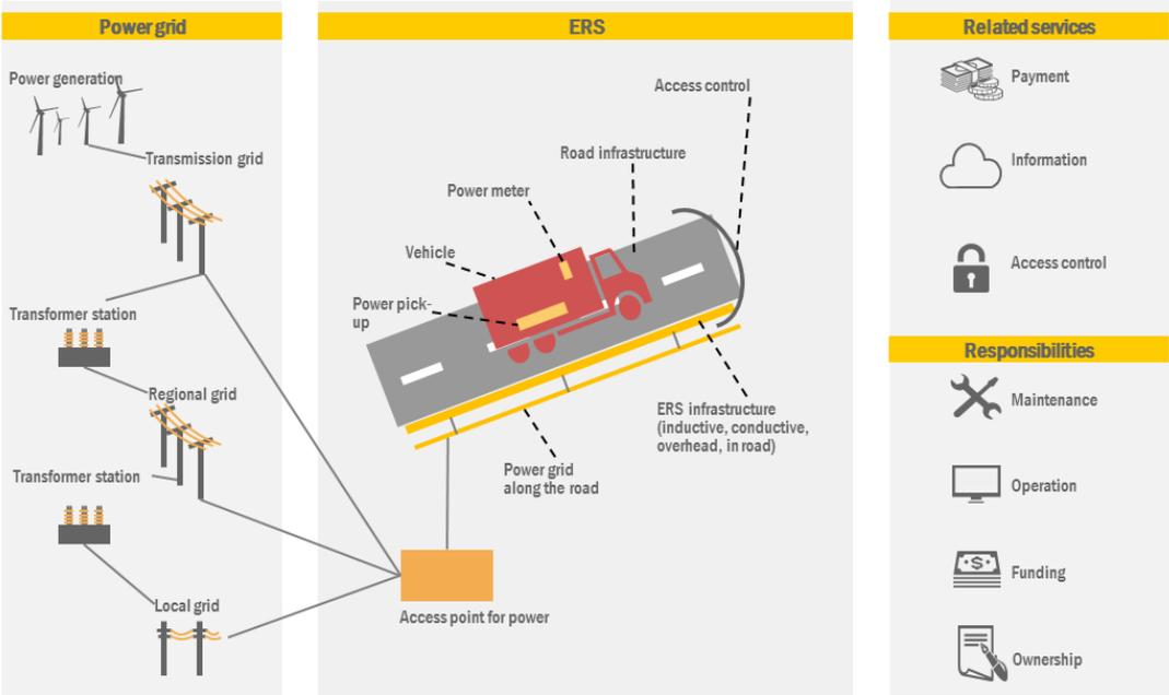
**Figure 2 – Principal layout of the electric road system and adjacent system and services**
