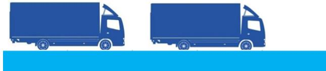
**Figure 4: 2-platoon on bridge category 1 ( $L=20\text{-}50\text{ m}$ , the truck represents all sorts of trucks including truck-trailers, the blue beam represents the bridge)**
