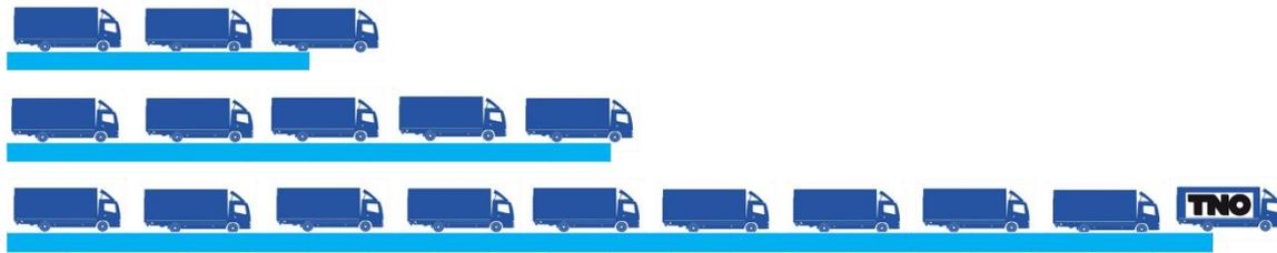
**Figure 1 – From top to bottom a category 1, 2 and 3 influence length with the maximum number of trucks (16.5 m) and spacing of 5 m. The picture of the truck does not (necessarily) represent the actual truck type.**
