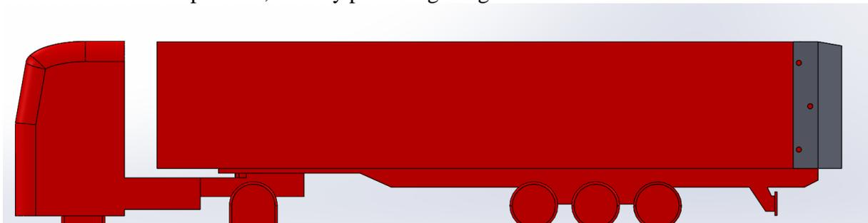
**Figure 1 – CAD drawing of simplified vehicle model with tail**
