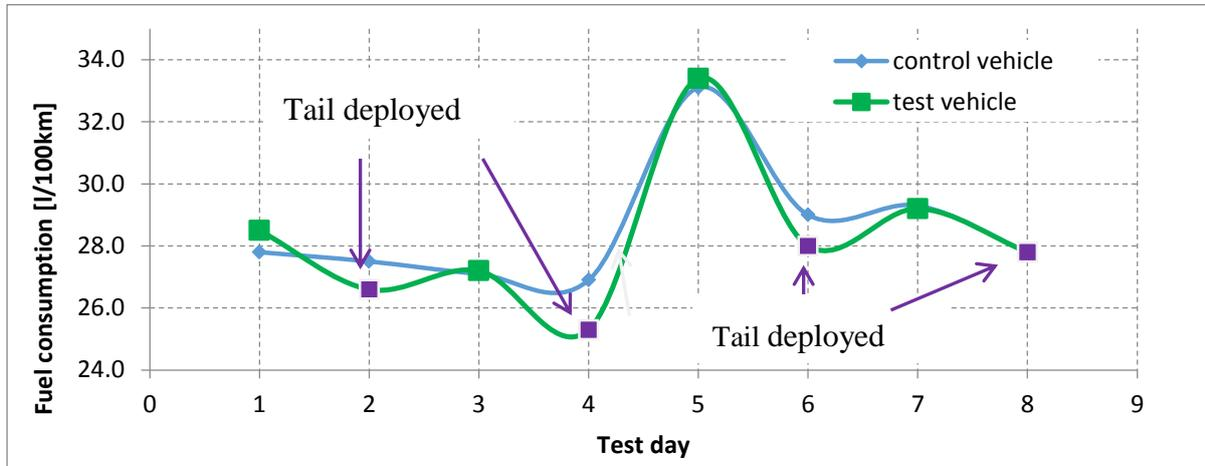
**Figure 8 - Measured fuel consumption during Operational test 1**
