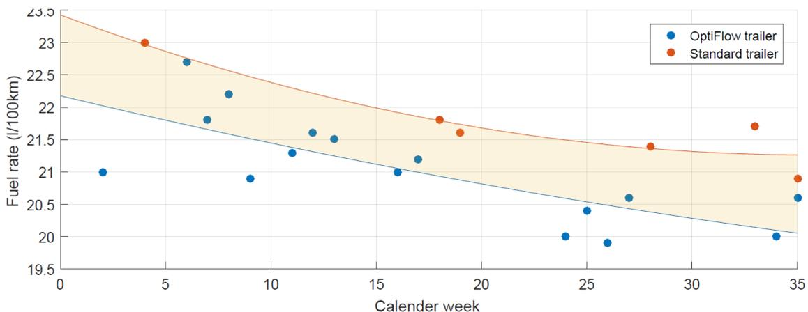
**Figure 9 - Measured fuel consumption during Operational test 2**
