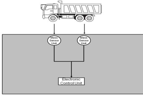
**Figure 1: Rigid Vehicle with OBM System**
